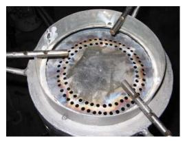
Figure 45. The Fabricated Gas Burner.
