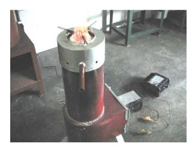
Figure 20. The CPU Proto-Type IDD/T-LUD Rice Husk Gas Stove Model 2.
