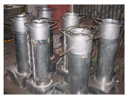
Figure 59. Completely Fabricated Six Units Rice Husk Gas Stoves.
