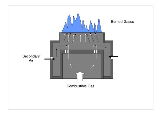
Figure 11. The Principle of the Burner Operation of the Rice Husk Gas Stove.
