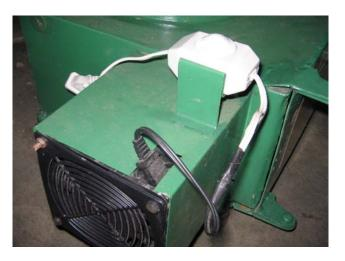
Figure 61. The Fan and the Switch Installed in the Stove.
