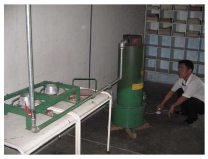
Figure 83. The Table-Top Multiple "Remote Burner" RHGS
