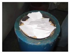
Figure 72. Placing Small Pieces of Paper on the Fuel Column.
