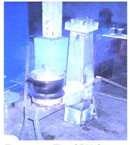
Figure 21. The CPU Cross-Flow Rice Husk Gasifier Stove.
