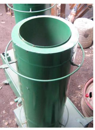
Figure 6. The Gasifier Stove Reactor.
