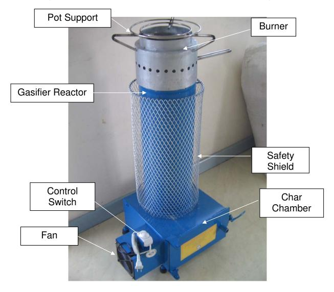
Figure 4. The Rice Husk Gas Stove Showing Its Various Parts.
