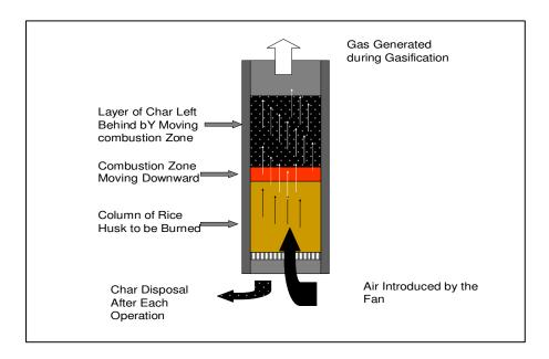
Figure 10. Schematic Drawing of the Principle of Operation of the Rice Husk Gasifier Reactor.
