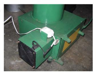
Figure 8. The Fan Assembly.
