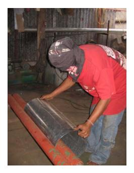
Figure 56. Forming Cylinders on Pipe Bender.
