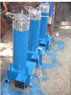
10. Install the fan and the electrical switches (Fig. 61) and check whether or not they are functioning properly. Make sure that the fan is properly bolted to the housing assembly. It should be carefully fixed into the housing without damaging the impeller so that it will minimize power loss during operation. The switch for the fan must be connected in series with the wire.
