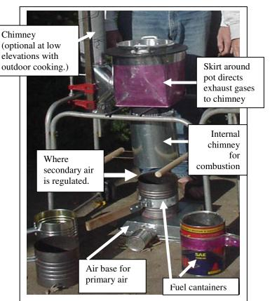
Figure 27. An improved Juntos Model B T-LUD gasifier stove, including chimney needed for altitudes above 1000 meters.
