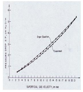
Figure 39. Pressure Draft of Rice Husk at Different Superficial Velocity of Gas.
