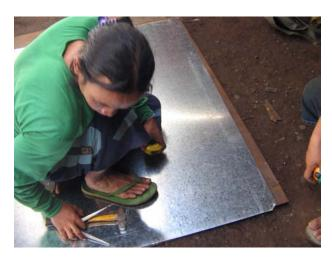
Figure 54. Layouting of Stove Parts.
