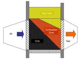
allows a continuous Cross Draft Type Rice Husk Gasifier operation of the Figure 37. Cross Draft Type gasifier reactor even whe Rice Husk. Gasifier.
