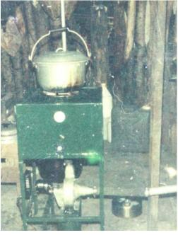
Figure 17. The CPU Single-Burner Rice Husk Stove.
