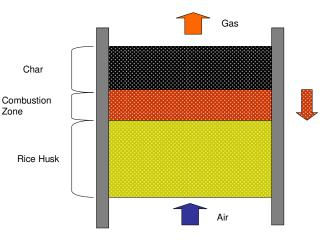
Figure 36 B. Inverted DownDraft Type Gasifier is Top-Lit with UpDraft
