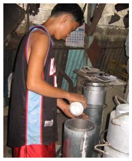
Figure 58. Filling Up of Rice Husk Insulation.
