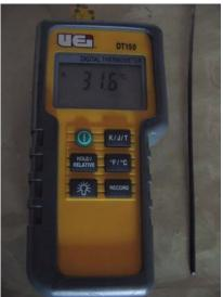
Figure 67. The Thermocouple Wire Thermometer.
