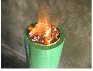
Figure 47. Firing Fuel on Top of the Reactor .
