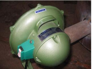
Figure 43. AC 220 Volt-1 Amp Centrifugal Blower.
