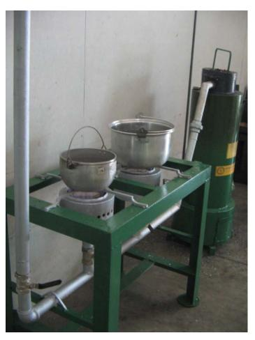
Figure 80. The Table-Type Multiple "Remote Burner" Rice Husk Gas Stove.
