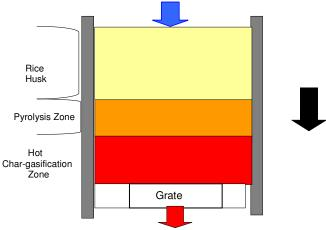
Figure 36 A. DownDraft Type Gasifier. (Bottom-Lit)
