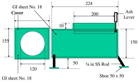
Longitudinal View of the Ash Chamber
