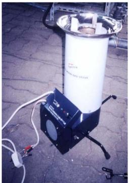
Figure 24. The Sri Lanka Wood Gas Stove.
