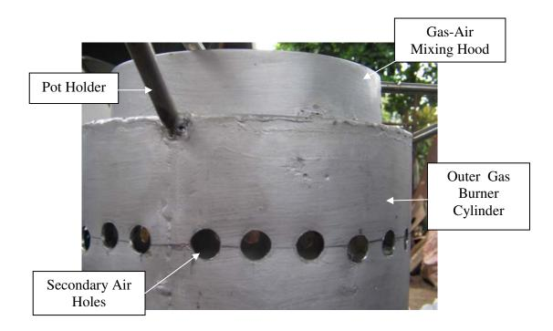
Close Up View of the Secondary Air Inlet Holes
